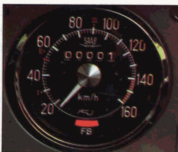
Red warning lamp for brake circuit failure
