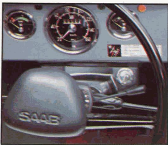
Lever for horn/windscreen wipers/windscreen washers
