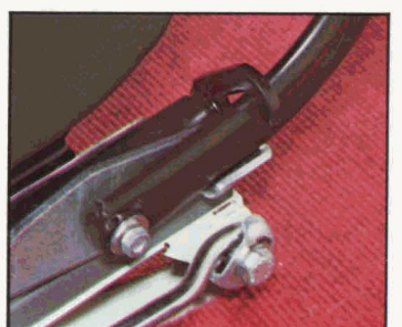
Catch to prevent passenger seat from tipping forwards
