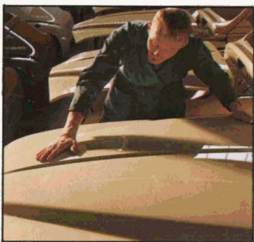
Control of paintwork
